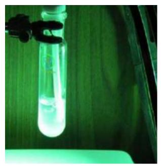
After bubbling ozone through cyclohexane illuminated with a UV lamp for a few hours adipic acid began to precipitate out © Science/AAAS
